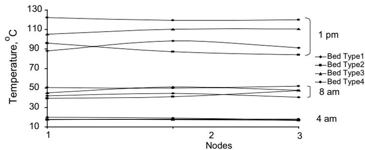
Fig. 6. Temperature distribution inside the four types of bed techniques at different times of heating (February).
