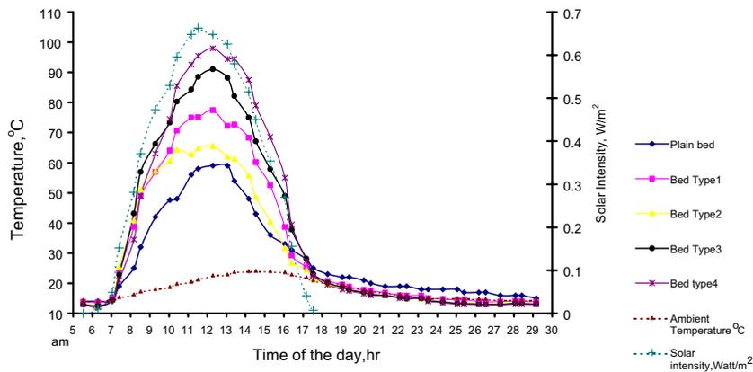
Fig. 5. Measured average temperature of the four types of bed techniques (February).
