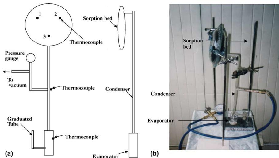
Fig. 3. (a) Modified glass tube, (b) photograph of the modified glass tube.
