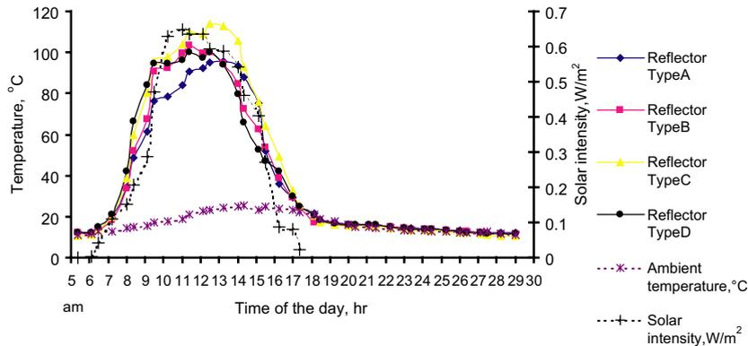
Fig. 7. Effect of reflector arrangements on the temperature of bed Type 4 (February).
