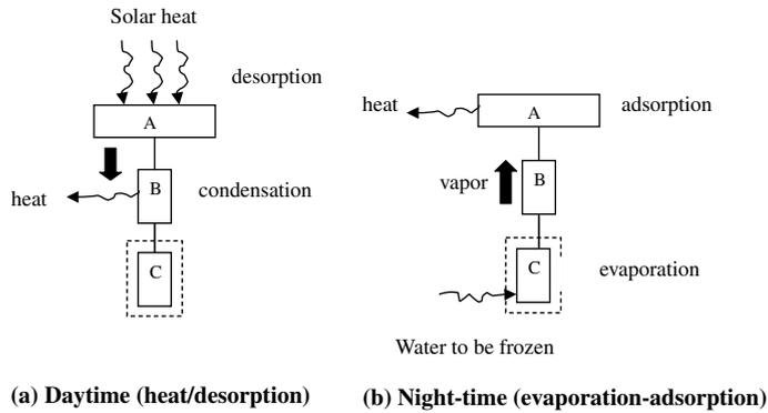
Fig. 1. Operation principle of solid adsorption refrigeration system utilizing solar heat. A: Sorption bed (solar collector); B: condenser; C: evaporator.
