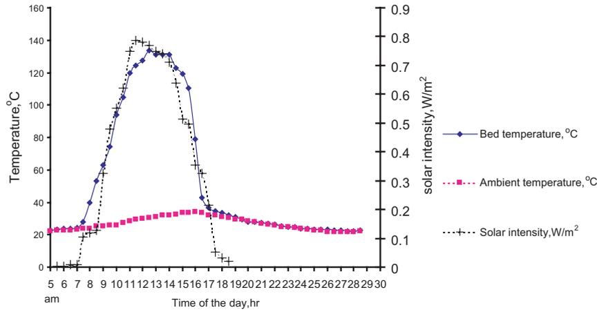
Fig. 9. Temperature of bed Type 4 when heated by reflector Type C (June).
