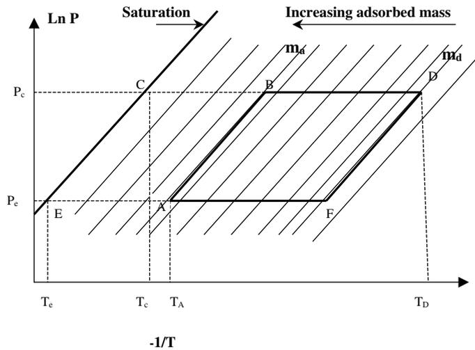
Fig. 2. Clapeyron diagram ( $\ln P$  versus  $-1/T$ ) of ideal adsorption cycle.
