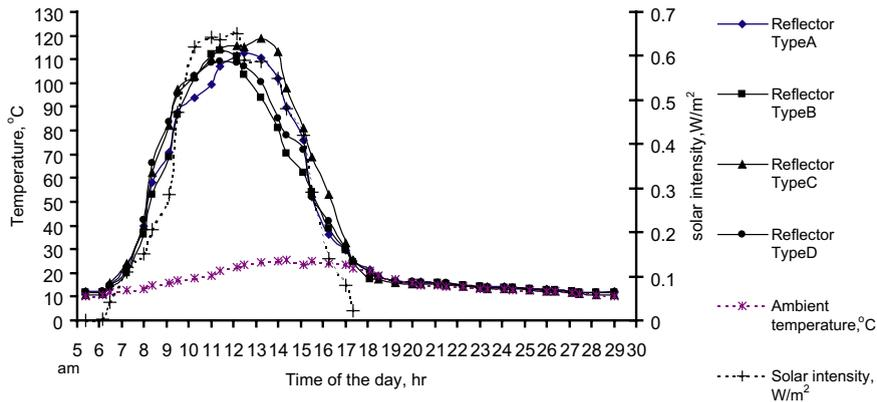
Fig. 8. Effect of using glass shell on bed temperatures Type 4 for different of reflector arrangements (February).
